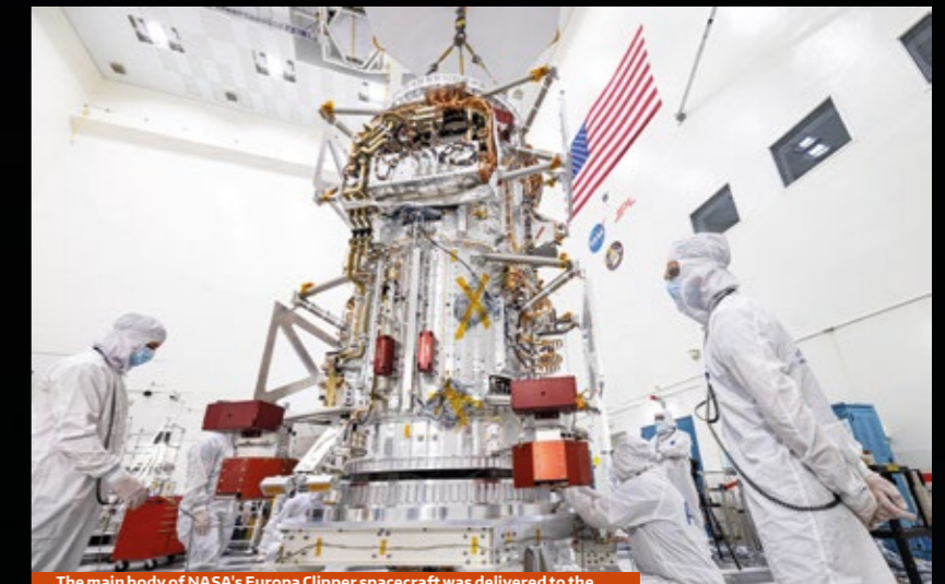
The main body of NASA's Europa Clipper spacecraft was delivered to the agency's Jet Propulsion Laboratory in Southern California, where engineers and technicians finished assembling the craft by hand before testing it (Courtesy of NASA/JPL-Caltech/Johns Hopkins APL/Ed Whitman)
